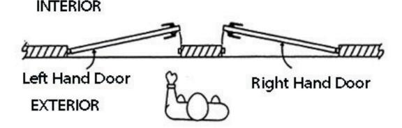
To determine hand, stand on the outside (or less secure) side of the door. While facing the door, if the hinge is on the right side of the door, the door is "right handed"; or if the hinge is on the left, it is "left handed".
