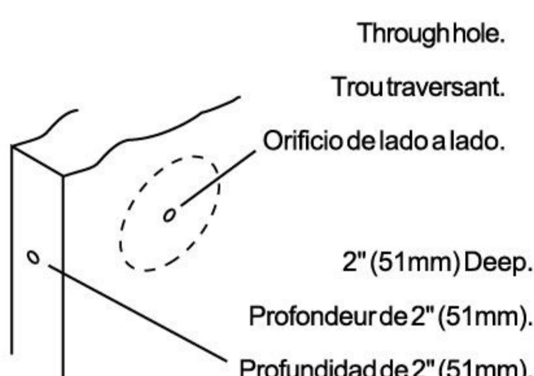
**C.** Drill the 2-1/8" (54mm) hole about halfway through door, then finish drilling from the other side to prevent splintering.
